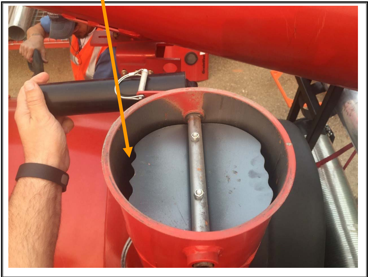
Figure 2 – Air Throttle Butterfly – Not Properly Installed
