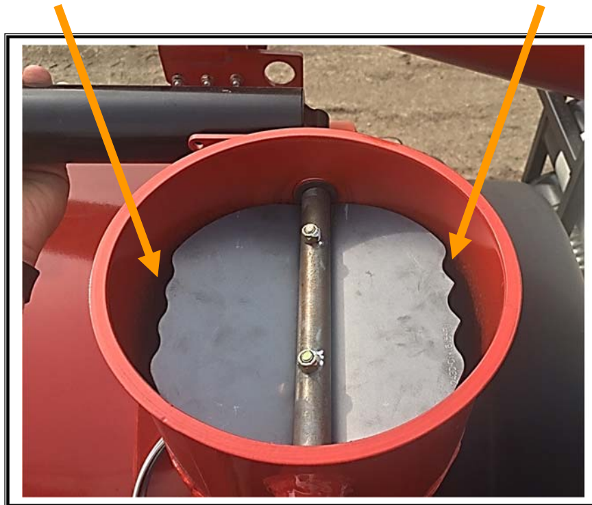
Figure 1: Air Throttle Butterfly – Properly Installed
