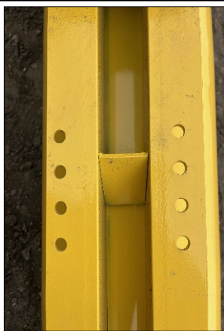
Figure 1 Off centered punched holes on track stop
